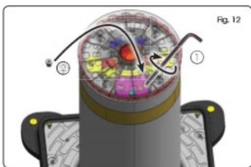
The closing screw on the bollard head can also be tightened upside-down to prevent access to manual hydraulic lowering. This operation has to be performed, of course, after having removed the head by unscrewing the 4 securing screws (see fig. 13 ref. ①)
